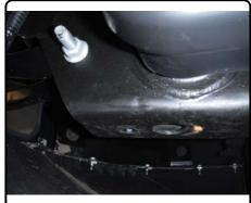
2. Fishwire the 1/2" carriage bolts and spacers into position through either the side of the frame, the end of frame, or the opening in the bottom of the frame. Do not pull bolts out through the frame so as to allow the hitch to move into position.
