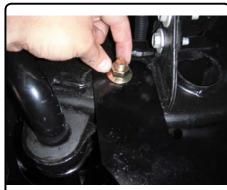
5. Torque all 1/2" fasteners to 110 lb-ft and all 12mm fasteners to 92 lb-ft.
