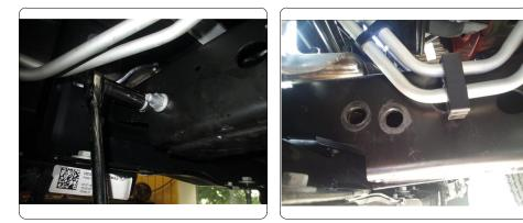
2. Fishwire (2) bolt plates removed in STEP 1 through original holes on inside of frame rails.
