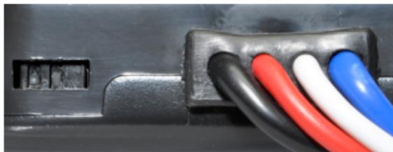
In the illustration above the switch on the right controls the level of output available to the trailer brakes when using the manual control. The factory default setting is the "ON" position with the switch down. This setting limits the manual control output to the level set using the output control thumbwheel. Moving this switch up to the "OFF" position allows 100% of the output to the brakes when the manual control is actuated regardless of the output control setting.
