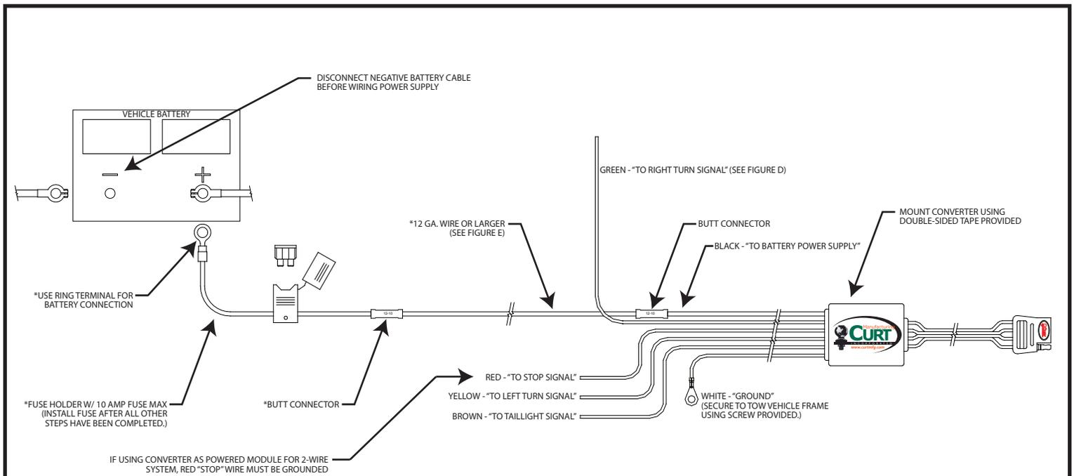
THIS CONVERTER SYSTEM IS TO BE USED ONLY ON 12 VOLT NEGATIVE GROUND SYSTEMS (ILLUSTRATION NOT TO SCALE)
