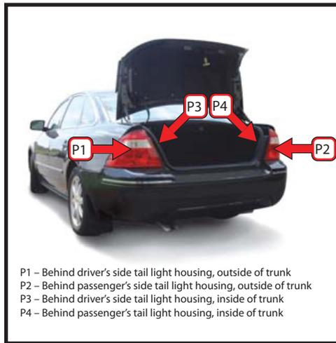
P1 - Behind driver's side tail light housing, outside of trunk
