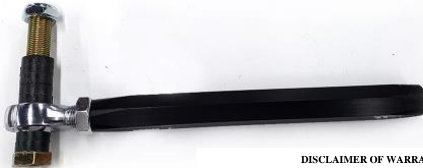
Figure 2: Adjusting Bump Steer with spacers
