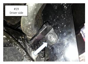
**Step - 9** Align the Winch bumper with the vehicle and tighten all factory and supplied nuts and bolts.
