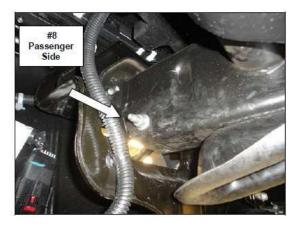
**Step-5** From the tow hook opening, slide the vehicle attachment end of the passenger side upper bracket under the frame, rotate the bracket and align the holes in the bracket with the holes in the frame and reinstall the tow hook front bolt and nut, then the rear bolt. (**Photo 9 & 10**)
