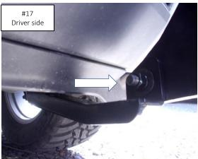
**Step-8** Hook the lower auxiliary bracket to the chassis **(Photo 18)**. Bolt the lower auxiliary bracket to the lower bracket using (1) carriage screw 3/8" (1) plain washer 3/8" (1) spring lock washer 3/8" (1) nut 3/8" **(Photo 19)**.
