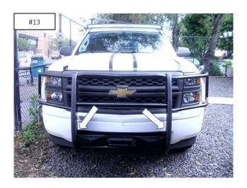
**Step - 7** Locate the hole in the bottom of the frame and install (1) 1/2" t-bolt, (**Photo 14 &15**). Attach the driver side lower bracket to the frame using the T-Bolt, (1) 1/2" flat washer, (1) 1/2" lock washer and (1) 1/2" hex nut, and to the Winch bumper using (1) 1/2" x 1 1/2" carriage bolt, (1) 1/2" flat washer, (1) 1/2" lock washer and (1) 1/2" hex nut, (**Photo 16 &17**). Repeat to install the passenger side lower bracket.
