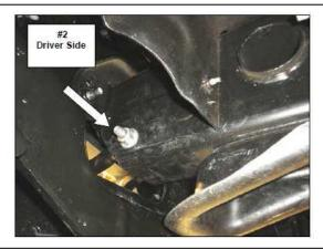
**Step-2** From the tow hook opening, slide the vehicle attachment end of the driver side upper bracket under the frame, rotate the bracket and position upper attachment hole in the bracket over the shank of the front tow hook bolt and reinstall the nut.
