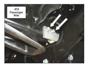
**Step-6** Place the center of the front hole in the driver and passenger side upper brackets approximately 8" from the bottom edge of the bumper cap, **(Photo 11)** and tighten all nuts and bolts securing the brackets. With assistance, position and attach the Winch Bumper to the outside of each upper bracket using (2) 1/2" x 1 1/2" carriage bolts, (2) 1/2" flat washers, (2) 1/2" lock washers and (2) 1/2" hex nuts, **(Photo 12&13)**. Leave the nuts and bolts loose for final adjustment.
