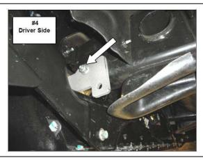
**Step-3** Attach the driver side auxiliary bracket to the side of the frame using the tow hook rear bolt and to the lower hole in the upper bracket using (1)  $\frac{1}{2}$ " x 1  $\frac{1}{2}$ " carriage bolt, (1)  $\frac{1}{2}$ " flat washer, (1)  $\frac{1}{2}$ " lock washer and (1)  $\frac{1}{2}$ " hex nut.(**Photo 5 & 6**).
