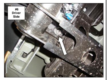
**Step-8** With assistance attach the bumper shell brackets to each frame bracket using (2)  $\frac{1}{2}$ " x 1  $\frac{1}{2}$ " hex bolts, (4)  $\frac{1}{2}$ " flat washers, (2)  $\frac{1}{2}$ " lock washers and (2)  $\frac{1}{2}$ " Hex nuts, Align the bumper shell with the vehicle, verify that the tailgate clears when lowered, and tighten all nuts and bolts, (Photo 7 & 8). If necessary loosen the frame / receiver hitch bolts to adjust the bumper replacement.
