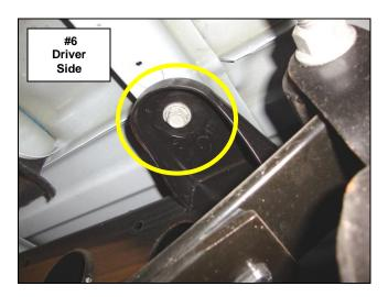
**Step-8** Remove the M10 bolt (1) per side and M14 bolts (2) per side securing the bumper brackets to the frame, (Photo 7).
