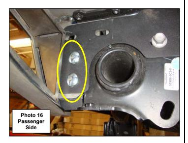
**Step-16** Align the replacement bumper with the vehicle, verify that the tailgate clears when lowered, and tighten all factory and supplied nuts and bolts.
