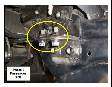
**Step-10** Position (2) of the round spacers between the extension bracket and frame, align the holes and reinstall the (2) factory bolts, (Photo 9 & 10). Snug but do not tighten the bolts. Repeat for the driver side.
