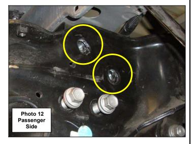
**Step-13** Remove the factory bolts and let the receiver hitch pivot and hang down. Using a rotary tool and bit to elongate the holes in each side of the receiver hitch, (Photo 13).
