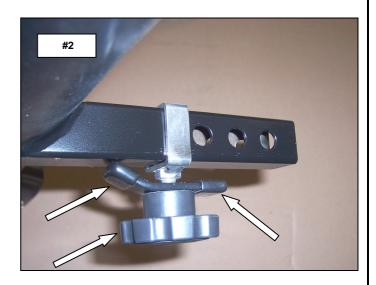
**Step-3** Insert the HitchStep receiver tube into the vehicle hitch receiver at the desired position. Align the holes in the HitchStep receiver tube with the holes in the hitch receiver and install the hitch pin and clip. Position the anti-rattle bracket underneath the hitch receiver opening and hand tighten the knob. **Photo** #3
