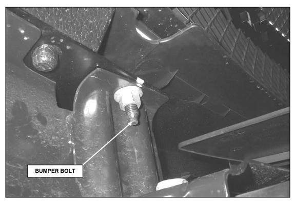
**STEP-2** BEGINNING WITH THE DRIVER SIDE, REMOVE THE NUT AND UPPER BUMPER BOLT. THE BOLT IS LOCATED ON THE BACK EDGE AT THE TOP OF THE BUMPER. THIS LOCATION WILL SERVE AS THE UPPER BRACKET MOUNTING POINT.
