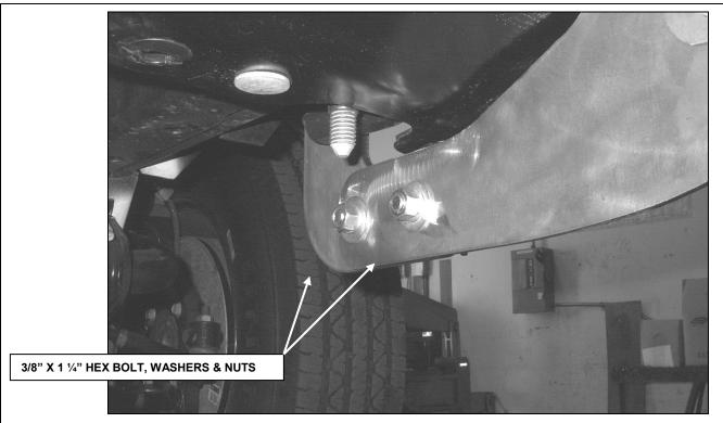
**STEP-8** ATTACH THE GRILLE GUARD ASSEMBLY TO THE LOWER BRACKETS, USING THE 3/8" x 1 1/4" HEX BOLTS, LOCK WASHERS, FLAT WASHERS AND HEX NUTS.
