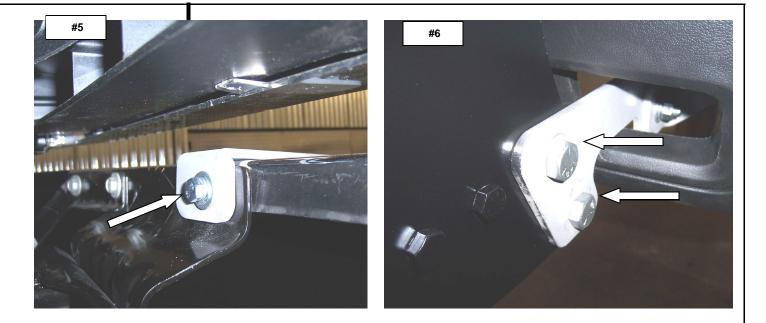
**STEP 7.** ATTACH THE GRILLE GUARD ASSEMBLY TO THE UPPER BRACKETS USING (2) 3/8" X 1 1/4" HEX BOLTS, FLAT WASHERS, LOCK WASHERS AND HEX NUTS. **PHOTO #7**
