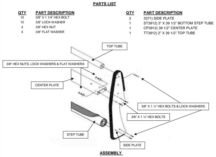
READ THE ASSEMBLY AND INSTALLATION INSTRUCTIONS COMPLETELY BEFORE YOU BEGIN. NOTE: THIS INSTALLATION REQUIRES CUTTING OR REMOVAL OF THE AIR DAM.
