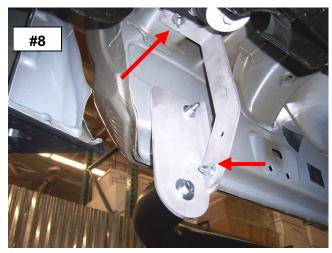
**STEP-9** ATTACH THE DRIVER SIDE STEP TO THE FRONT AND REAR BRACKETS USING (1) 1/2" X 2" HEX BOLT, (1) ½" FLAT WASHER AND (1) 1/2" LOCK WASHER FOR EACH BRACKET.
