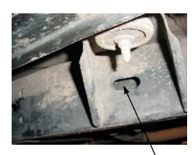
Introduce here a 1/2 x 1 1/2" cut carriage head bolt
