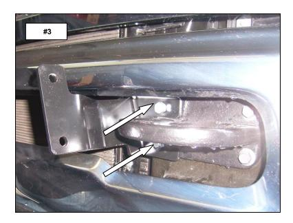
**STEP-3** POSITION THE RHINO CHARGER BULL BAR MOUNTING TABS BETWEEN THE DRIVER AND PASSENGER SIDE BRACKETS AND ATTACH THE TABS TO THE BRACKETS USING (2) 3/8" X 1" HEX BOLTS, FLAT WASHERS, LOCK WASHERS AND HEX NUTS. **PHOTO #4**
