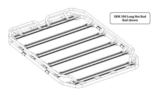
• **Step-4** Align the rails and fully tighten all hardware and continue the SRM roof rack installation.
