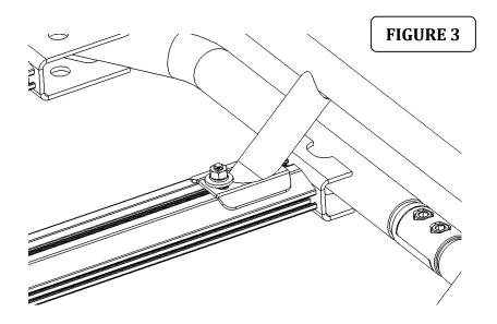
**Step-3** Secure the rail to the bolts installed using (1) 1/4" flat washer, (1) 1/4" lock washer and (1) 1/4" hex nut, per bolt (Fig 3). Do not tighten the bolt.
