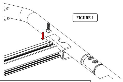
**Step-1** Install (1) 1/4" x 3/4" hex bolt for every rail bracket in the channel of every crossbar that will be facing up the rail plates. (Fig 1).
