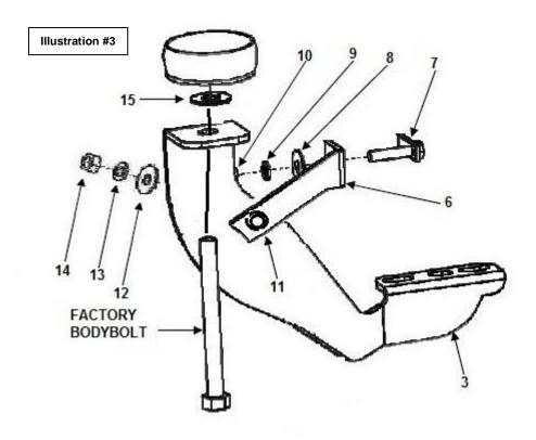
**Step-7** Attach the passenger side step to each of the brackets using (2) 5/16" x 1" hex bolts, (2) 5/16" lock washers and (2) 5/16" flat washers, **(Photo 7)**.
