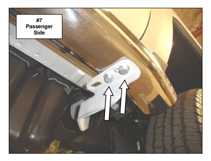
Step-8 Align the side step with the vehicle and tighten all side step and bracket nuts and bolts, (Photo 8).
