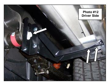
**Step-5** Re-align the side bar with the vehicle and tighten all side bar, bracket and vehicle nuts and bolts.
