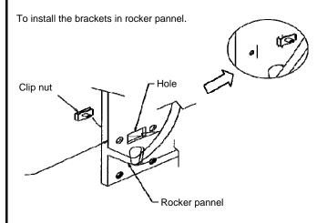
3. Mount bracket and attach with: (1) 3/8 x 1 1/4" hex head bolt, (1) 3/8" flat and lock washers, in lower part attach with: (1) 3/8 x 1 1/4" hex head bolt, (2) 3/8 flat washer, (1) 3/8" lock washer, (1) 3/8" hex nut. **SEE ILLUSTRATION 4.** By each bracket. Leave loose.
