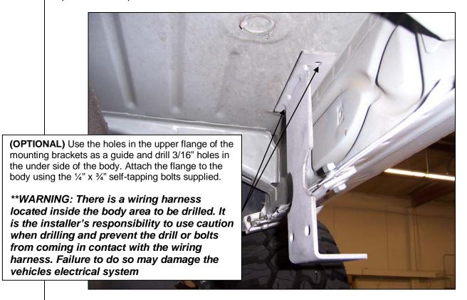
**Step 4**. Loosely attach the flange of the mounting brackets to the bottom of the lower body pinch mold using the 3/8" x 1" hex bolts, flat washers, lock washers and nuts as shown.
