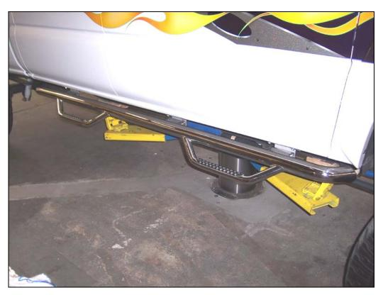
**Step 6.** Align sidestep with the body and then tighten all mounting bracket and sidestep nuts and bolts. **Step 7.** Repeat the above installation steps to install the driver side mounting brackets and sidestep.
