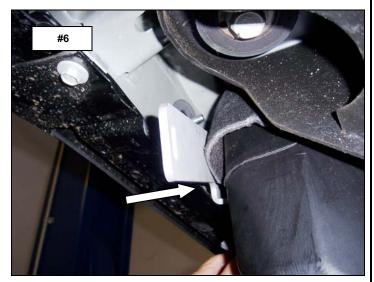
**Step-4** Position the hole in the front of the bracket over the T-Bolt and install (1) 3/8" flat washer, (1) 3/8" lock washer and (1) 3/8" hex nut. Align the hole in the flange of the bracket with the U-Nut and install (1) 5/16" flat
