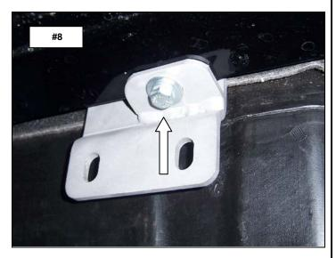
**Step-5** Passenger side Center bracket installation.
