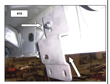
**Step-6** Passenger side rear bracket installation.
