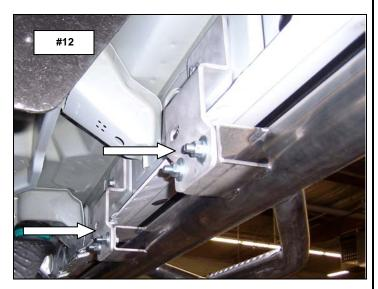
Step-8 Align the side step with the vehicle and tighten all nuts and bolts.
