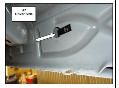
**Step-4** Attach one of the driver side brackets to the rocker panel using the U-Nut, (1) M8 hex bolt, (1) 5/16" lock washer and (1) 5/16" flat washer, and to the pinch mold using (1) M8 hex bolt, (2) 5/16" flat washers, (1) 5/16" lock washer, and (1) M8 hex nut. Leave the nut and bolts loose for final adjustment, **(Photo 8)**.
