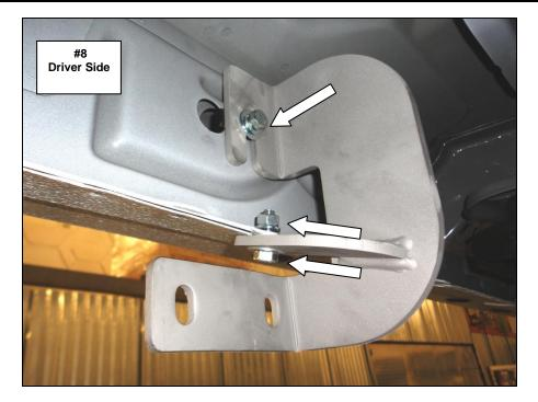
**Step-5** Install the driver side rear bracket by measuring from the front fender bolt reward approximately 75 1/8" and repeat the above steps.
