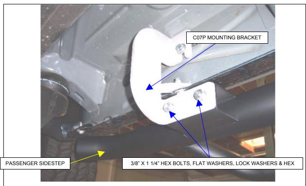
**STEP 6.** Position the passenger sidestep up to the vehicle and loosely attach it to the mounting brackets using the 3/8" x 1 1/4" hex bolts, flat washers, lock washers and hex nuts.
