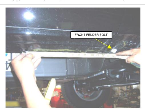
**STEP 2.** This installation uses three mounting brackets per side. Begin by installing the passenger side front mounting bracket. Measure reward from the front fender bolt approximately 14" and locate the single hole in the body pinch mold and the square nut spot welded in the rocker panel.
