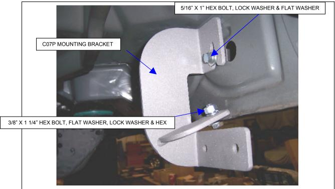
**STEP 5.** Loosely attach the two remaining C07P mounting brackets to the rocker panel and pinch mold using the 5/16" and 3/8" fasteners as shown.
