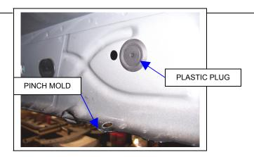
**STEP 4.** Locate the holes in the body pinch mold and rocker panel for the center and rear mounting brackets. Measure rearward from the front fender bolt approximately 58 7/8" for the center and 75 1/8" for the rear bracket. Remove the plastic plugs from the rocker panel and install 5/16" U-NUTS in the rocker panel as shown.
