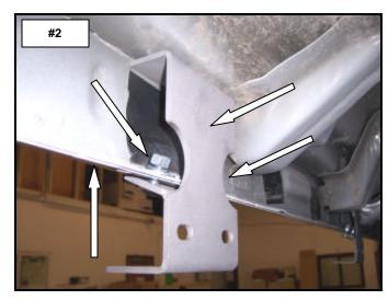
**STEP 2.** ATTACH EACH OF THE MOUNTING BRACKETS TO THE PINCH MOLD USING (2) 3/8" X 1" CARRIAGE BOLTS, (2) FLAT WASHERS, (2) LOCK WASHER AND (2) HEX NUTS. HAND TIGHTEN. **PHOTO'S** #2 & #3
