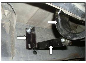
Shows the central bracket assembly. Picture passenger side.
