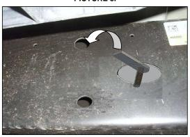
Insert the 3/8" threaded rod plate in the hole as shown. Place the middle auxiliary bracket A and attach whit 3/8" bolts.
