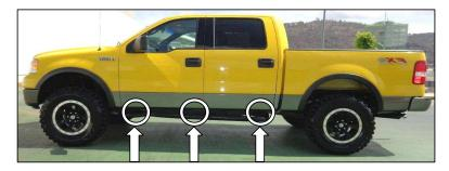
In this part, install each bracket on driver side.
