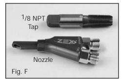
where you want to mount the nozzle, tap the hole and install the nozzle. Once the nozzle is installed, place the appropriate tuning jets in the nozzle and attach the 2-foot long, -3AN hoses to the nozzle jet fittings and the Nitrous Management Unit (Fig.G).
