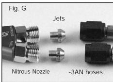
\*Note: Ensure that the fuel connection on the Nitrous Management Unit is connected to the fuel jet fitting on the nitrous nozzle. Ensure the same for the nitrous connections.
