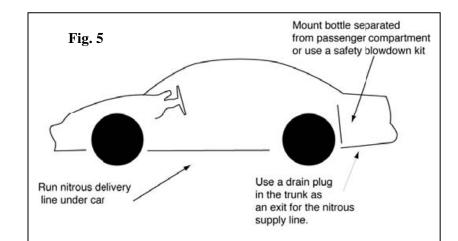
**3.** Mount nitrous delivery line under the car - When routing the nitrous delivery line under the car, try to use the subframe as a conduit (Fig. 5). This protects the line and eliminates the need to use clamps. The supplied cable ties work if you can run the line higher in the under-body so that it's safe from the road level obstacles such as speed bumps. For the pro-race look, you can use steel loom clamps with rubber sheathing to fasten the line to the body.
