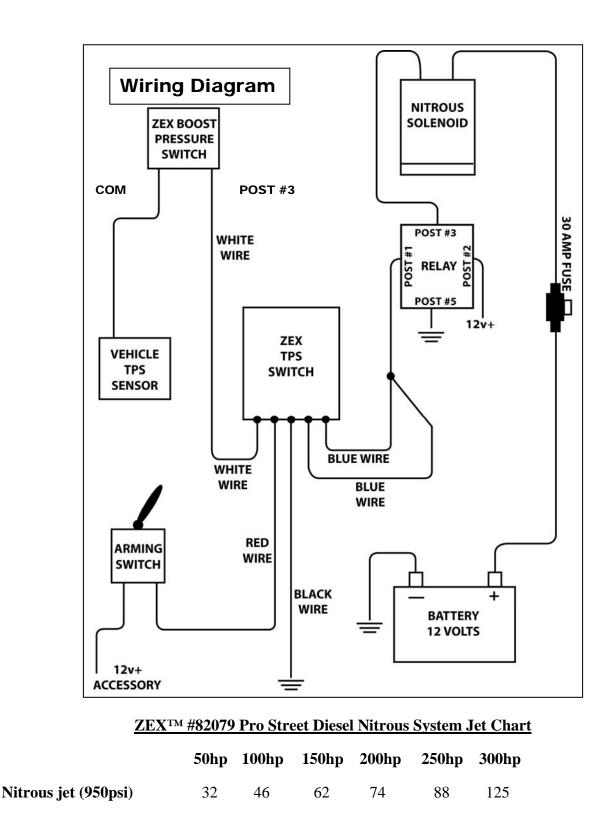
Note: Remember, a nitrous jet's power rating is the maximum amount of additional power it can support, it must have additional fuel tuning to achieve its maximum rated power.
