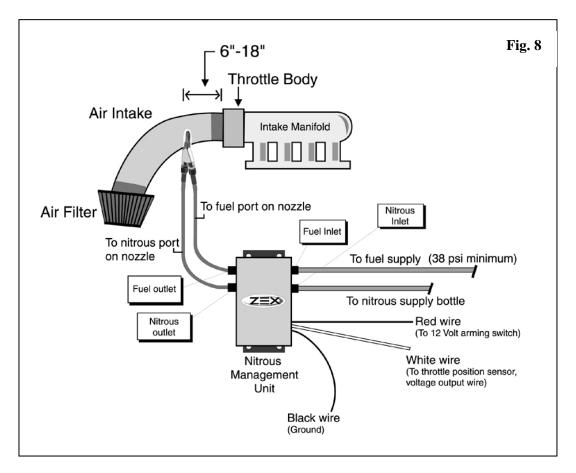
B. Take the black wire that comes from the Nitrous Management Unit and attach it to a suitable chassis ground. Remember to remove any paint at the attachment point to ensure a good ground.
