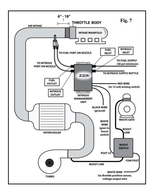
**6. Install boost pressure switch.** Locate the rubber line that connects your turbo's wastegate pressure fitting to the manifold pressure fitting. Cut this rubber line and install the boost pressure switch "in-line". Secure the rubber hose ends that have been slipped over the boost switch's hose barbs with a couple plastic tie straps.
