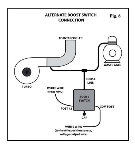
The Boost Pressure Switch is adjustable from 2-24psi, but is factory set at 7psi. Adjustments can be made using the 5/64 Allen screw located on the boost switch itself. Clockwise will increase the boost activation point and counterclockwise will decrease the boost activation point.
