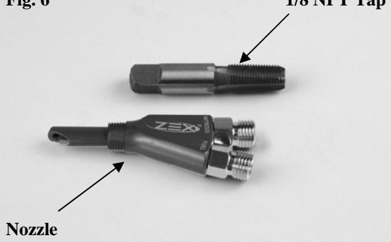
the spray is in the direction of airflow. We've also enclosed a tap (Fig. 6) should you desire to mount the nozzle directly into a metal air intake tube. Just drill an 11/32 inch hole where you want to thread-in the nozzle, tap the hole and install the nozzle. Once installed, place the appropriate tuning jets in the nozzle and attach the 2-foot long, -3AN hoses to the nozzle jet fittings and the Nitrous Management Unit (Fig.5).
