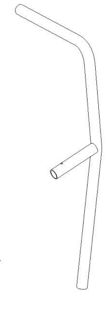
**Step 7:** Position hinge bracket as shown @ 1 5/8", and tack weld.
