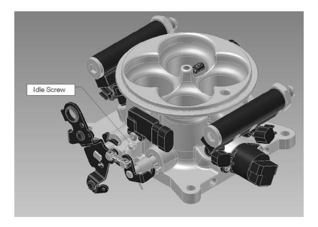
• **TPS IDLE RE-CALIBRATION.** The throttle position sensor is connected to the throttle shaft. So adjusting the resting position of the throttle blades in the previous step may have changed the voltage the ECU is receiving from the TPS. To account for this, you will again be asked to leave the throttle at the idle / closed position and let the ECU capture that voltage.
