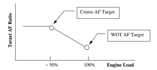
Just as the Cruise AF target can be adjusted for fuel economy, the WOT AF target can be adjusted for maximum power. It is quite possible that the engine can make more power at an air/fuel ratio that is leaner (higher number) than the preloaded WOT AF target. Or it might prefer a richer (lower number) air/fuel ratio. This is less likely, but it all depends on the engine.
