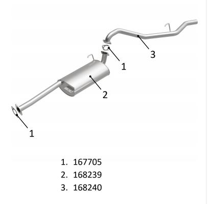
(Carefully read all instructions before installation) Disconnect the vehicle's battery before removal of the OEM exhaust system. This will prevent electrical accidents and will reset the computer if it applies to the vehicle. Remove existing exhaust system from the vehicle. Only remove parts that will be replaced. Clean existing flange with a wire brush to ensure proper sealing.
