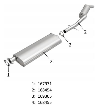
(Carefully read all instructions before installation) Disconnect the vehicle's battery before removal of the OEM exhaust system. This will prevent electrical accidents and will reset the computer if it applies to the vehicle. Remove existing exhaust system from the vehicle. Only remove parts that will be replaced. Clean existing flange with a wire brush to ensure proper sealing.
