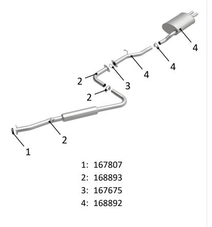
(Carefully read all instructions before installation) Disconnect the vehicle's battery before removal of the OEM exhaust system. This will prevent electrical accidents and will reset the computer if it applies to the vehicle. Remove existing exhaust system from the vehicle. Only remove parts that will be replaced. Clean existing flange with a wire brush to ensure proper sealing.
