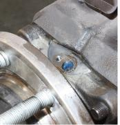
18MM - Behind the knuckle, you'll find the 4 bolts that retain the axle/hub assembly. Remove these bolts.
