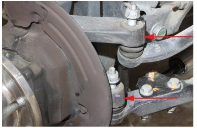
10. 18MM - Behind the knuckle, you'll find the 4 bolts that retain the axle/hub assembly. Remove these bolts.
