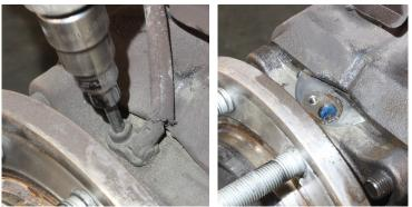
9. 21MM - Remove Drag Link and Tie-Rod from Passenger's side knuckle connection points. We back these nuts off until they're only engaged a few threads then strike the knuckle housing - see arrows below - (NOT the tie-rods) with a hammer under the joint drops. Then remove the nut and linkage.
