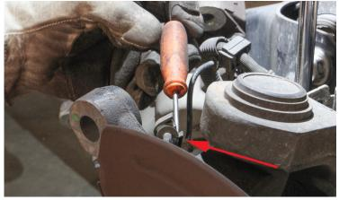
8. 5MM Allen - GENTLY Remove the ABS Sensor from the hub
