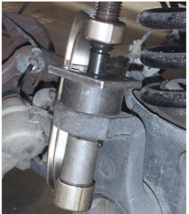
b. The Lower presses out from the bottom. No specific specification of press cups are used for this, the lower cup must be larger than the OD of the ball joint and deep enough to allow the ball joint to be pressed all the way out (*The OTC Large Cup/Plate would work* great on the bottom). We put the press directly on the ball joint but a cup can be used to distribute the load if preferred.
