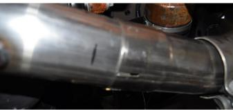
Slide the muffler inlet pipe over the passenger side X-Pipe outlet. NOTE: The use of a soap and water solution may aid in the installation of hanger grommets.
