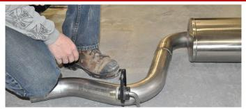
5. Locate the passenger side hanger grommet from Removal Step 5 and the passenger side muffler. Install the hanger grommet onto the front hanger of the muffler in the same position as previously installed on the stock exhaust. NOTE: The use of a soap and water solution may aid in the installation of hanger grommets
