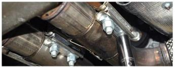
Use a 3/8" drive ratchet and 15mm deep socket, to loosen the two sleeve clamps at the cat-back connection point. Both nuts must be loosened in order for the clamp to fully disengage.
