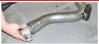
**6.** Locate one 3" clamp. Install the clamp on the passenger side muffler inlet pipe so that the bolt is vertical with the nut towards the ground and the bolt is towards the inside of the vehicle.
