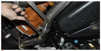
10. Tighten the clamp connecting the passenger muffler inlet pipe to the passenger side X-Pipe outlet using a ratchet and 15mm deep socket until muffler assembly is snug on the X-Pipe. Repeat Install Steps 5-10 on the driver side of the vehicle.
