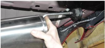
7. Slide the rear hanger into the rear hanger grommet located on the vehicle above and just inside of the passenger side tip cut out.
