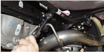
9. Locate the 13mm bolt removed during Removal Step 3 of the stock exhaust removal process. Install the front passenger hanger grommet assembly onto the rear suspension sub-frame and tighten it down with the 13mm bolt, using the 3/8" ratchet and 13mm socket.
