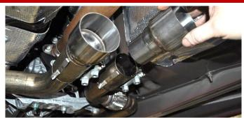
1. Locate the two X-Pipe inlet adapters. Slide the adapters into the factory sleeve clamps, and tighten using the ratchet and 15mm deep socket, until the adapters are snug in the clamps.
