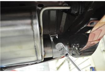
11. Locate the passenger rear tip assembly and one 3" clamp. Install the clamp on the tip inlet pipe so that the bolt is horizontal with the nut towards the inside of the vehicle and the bolt towards the top. Slide the tip assembly over the muffler outlet pipe and tighten the clamp using the ratchet and 15mm deep socket until the tip assembly is snug on the muffler outlet pipe. Repeat for the driver side tip assembly.
