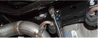
Use a 3/8" drive ratchet and 13mm socket, to remove the bolt holding down the driver side hanger grommet assembly.
