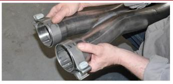
Install two 3" clamps on the driver and passenger inlets of the Double X-Pipe so that the bolts are vertical with the nut towards the ground and the bolts towards the outside of the vehicle.
