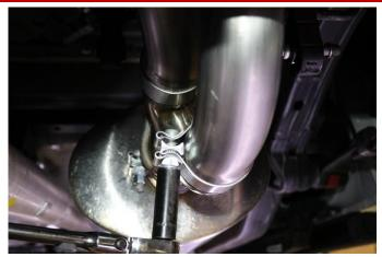
**16.** Snug the driver's and the passenger side front tailpipe TORCA clamps using a 15mm socket as shown. Make sure to leave the clamps loose enough to adjust position and rotation of the pipes.
