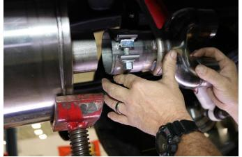
**9.** Slide the Y- Pipe Assembly into the side of the muffler supported by the stand as shown.
