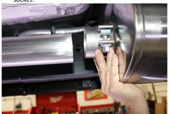
**5.** Slide the expanded end of the muffler into the headpipe.
