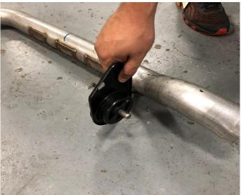
**14.** Remove the factory grommet from the passenger side tail pipe hanger and reattach it to the frame using a 13mm socket.
