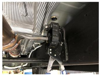
Remove the grommets from the Headpipe hangers at in the front of the muffler behind the flex pipe, using grommet pullers or similar device.
