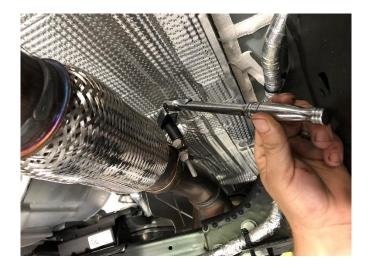
**3.** Use a 13mm socket to loosen the spherical clamp on the factory headpipe. Keep the factory spherical clamp for use with your Corsa Exhaust System.
