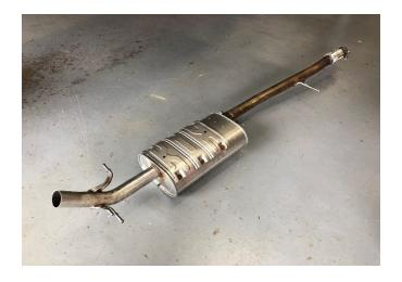
**7.** Remove the front section of the factory exhaust system and lay it aside.
