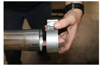
**17.** Insert a TORCA 2.5" clamp into the expanded and notched end of the passenger side rear tailpipe as shown.
