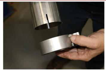
**8.** Insert a 3" TORCA clamp into the expanded and notched end of the Y – Pipe Assembly as shown.
