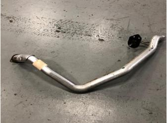
**10.** Carefully remove the driver's side tail pipe section.
