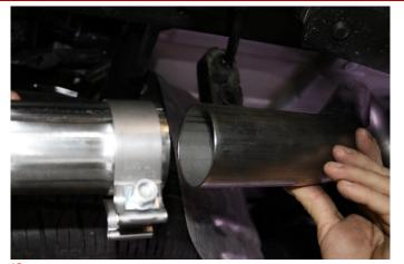
Slide the expanded and notched end of the passenger side rear tailpipe into the passenger side front tailpipe. Snug the TORCA 2.5" clamp using a 15mm socket.
