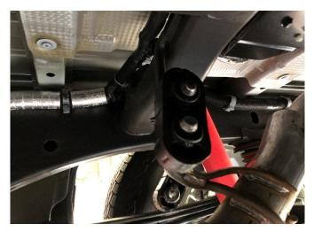
**5.** Remove the left grommet from the left tailpipe hanger at the muffler exit, using grommet pullers or similar device.
