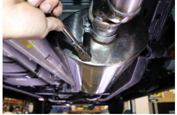
**11.** Snug the TORCA 3" clamp using a 15mm socket on the Y-Pipe Assembly as shown.
