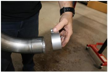
**14.** Insert a TORCA 2.5" Clamp into the expanded and notched end of the Passenger side Front Tail Pipe.
