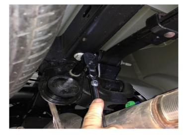
**9.** Disconnect the factory grommet from the frame using a 13mm socket on the driver's side tailpipe.
