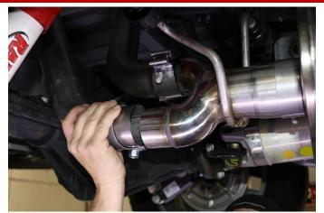
**15.** Slide the passenger side front tail pipe into the bottom section of the Y-Pipe as shown.
