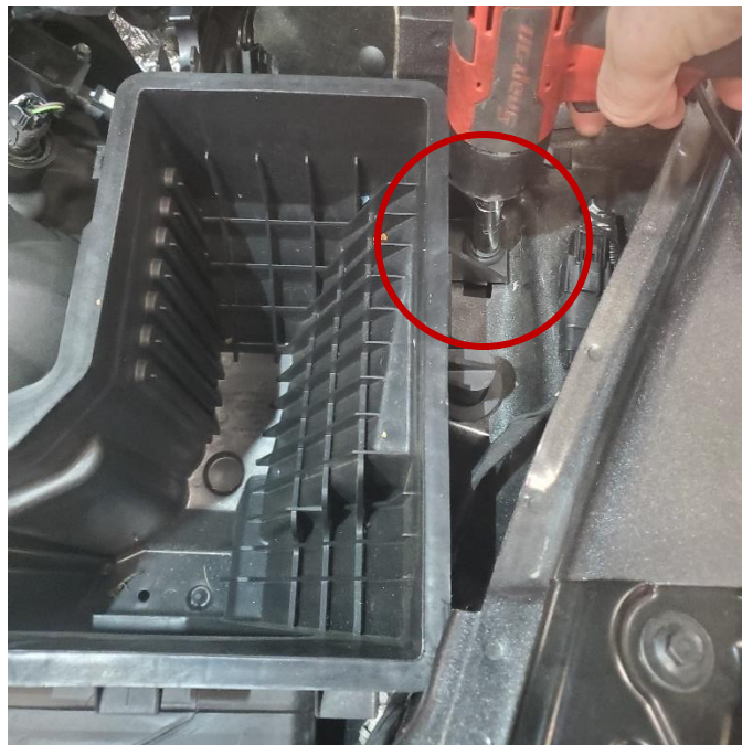
14. Remove 10mm bolt, then remove box from vehicle. Save bolt for installation.
