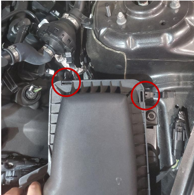
11. Undo two clips securing the upper airbox to the lower half.
