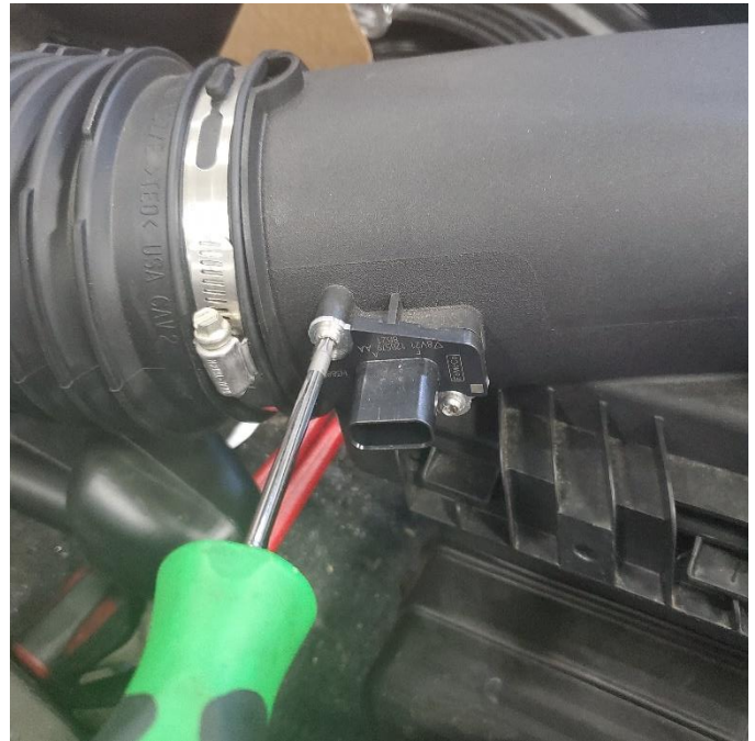
18. Remove MAF sensor from factory duct with T20 Torx driver.
