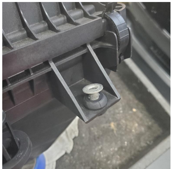
20. Remove metal bushing and rubber grommet from air box. Save for installation.
