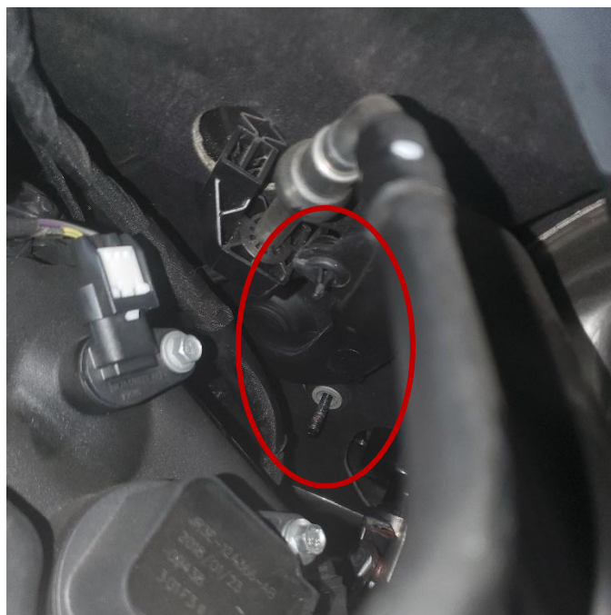
16. Remove 10mm nut with short wrench and unclip sound tube. Remove sound tube from vehicle. Install included plug to cover hole in firewall.
