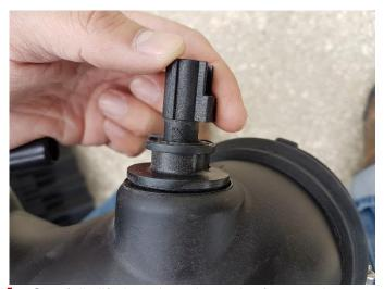
4. Carefully lift the tab and turn the factory air temperature sensor in the stock grommet to unclip it from the duct.
