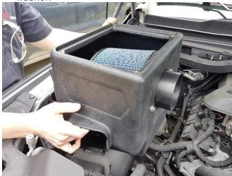
**8.** Align the four grommets in the Corsa box to the four mounting points in the car as shown.
