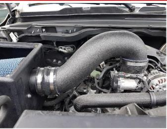
15. Slide the other end of the duct into the reducer on the throttle body then tighten all the clamps using a 8mm socket and ratchet.
