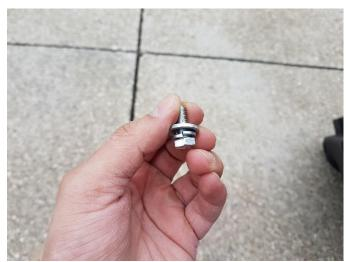
**6.** Assemble the included screw, washer and lock washer.
