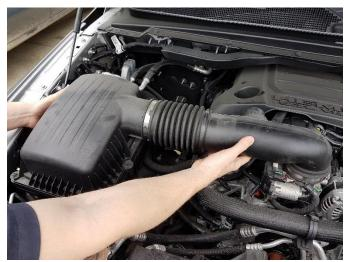
3. Loosen the stock clamp at the throttle body using an 8mm socket & ratchet and remove the stock intake by pulling up on the box and the duct.
