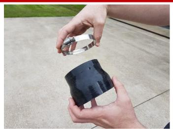
**10.** Install the 3.5" Clamp onto the small end of the reducer.
