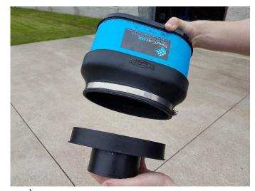
**3.** Insert the adapter into the filter (Maxflow 5 or Powercore).
