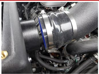
**14.** Install the last 4" Clamp onto the other end of the hump hose and slide the duct onto the box assembly.
