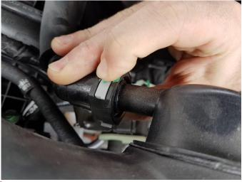
Disconnect the crank case vent hose by pressing the grey tab and gently pulling away.
