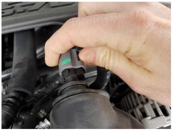
**1.** Disconnect the air temperature sensor harness from the stock intake tube.
