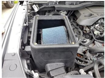
Press the box into the mounting points until fully seated.
