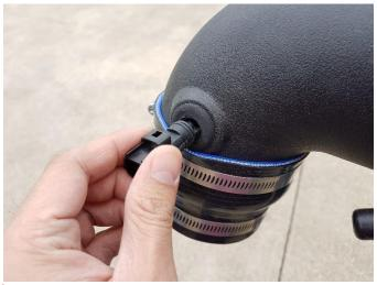
Carefully insert the stock air temperature sensor into the Corsa air duct. NOTE: The use of soapy water solution on the inside of the grommet might help to insert the sensor..
