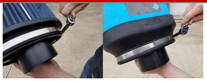
4. Tighten the clamp on the filter using a 8mm socket and ratchet.
