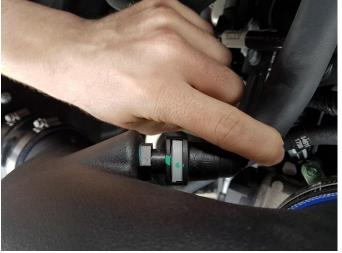
Connect the crank case vent hose to the fitting until it clicks.
