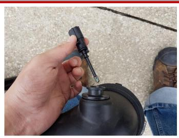
**5.** Gently remove the air temperature sensor from the factory air duct and keep it aside for installation of your Corsa Cold Air Intake.
