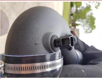
2. Turn the sensor such that the sensor clip for the harness is facing the arrow in the duct.
