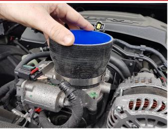
**11.** Install the reducer with the clamp onto the throttle body and tighten the clamp using a 8mm socket and ratchet.
