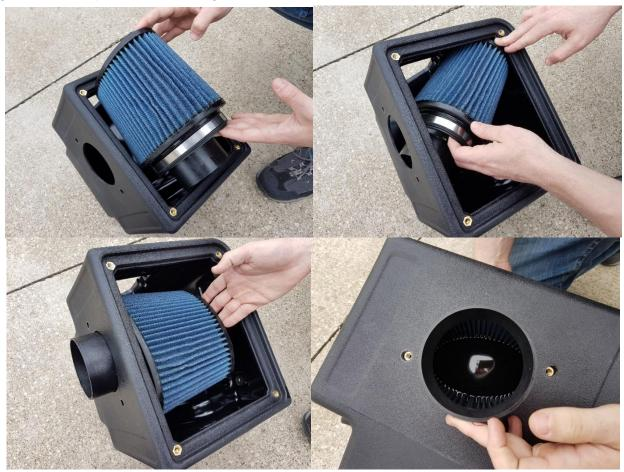
**5.** Insert the filter into the box and turn the filter adapter to align the holes on the box with the threads in the adapter.
