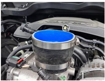
**12.** Place a 4" clamp onto the other end of the reducer.
