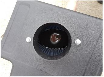
Secure adapter to airbox using a 10mm socket and ratchet.
