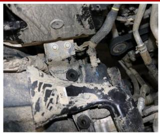
Locate the two factory grommets from removal step 9 and install them back into the factory location beneath the air box.
