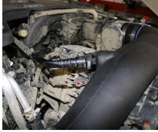
11. Connect factory breather hose to quick connect 12. Connect ATS wiring harness onto sensor. fitting in CORSA air duct.
