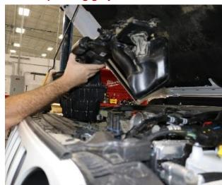
**8.** Lift complete factory air intake from vehicle as one assembly.
