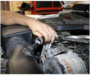
6. Disconnect the breather hose from the factory air duct by squeezing gray tab and pulling straight off.
