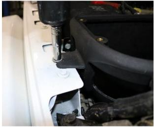
5. Locate the supplied mounting bracket and the factory bolt from removal step 5. Install the bracket from the inside of the air box under the tab. Install factory bolt through bracket with a ratchet and 10mm socket.
