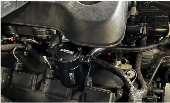
3. Align the hole on the catch can bracket to the bolt hole that secures the engine cover. When aligned, reinstall the engine cover and thread in the T-30 Torx bolt to the catch can. Reinstall other T-30 bolt to secure engine cover.
