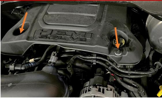
**1.** Remove the 2 bolts that secure the engine cover by using a T-30 Torx wrench. Pull engine cover towards the front of the vehicle to separate engine cover from rubber grommets to fully remove.
