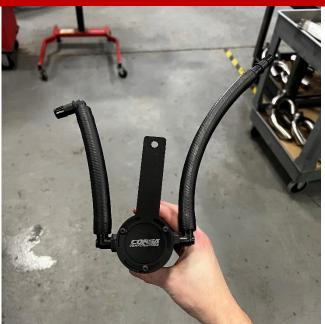
Install fittings with an 11/16" Wrench. Use a 2.5mm Hex wrench to secure bracket to the catch can. IMPORTANT: Corsa recommends using thread sealant or PTFE tape on barbed fittings and bottom drain plug to prevent any leaks.
