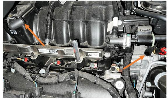
**2.** Remove factory PCV line from the passenger side of the vehicle in the 2 locations shown.
