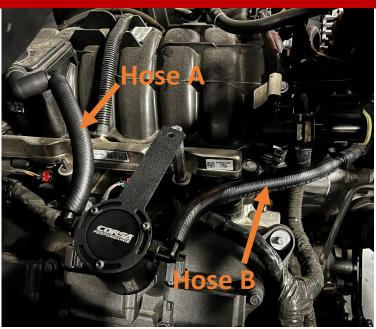
First connect the barbed fittings to the PCV hose ends. Make sure Hose A connects to the side located on top of the engine and Hose B connects to the side on the front of the engine.
