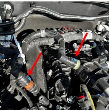
Remove the stock PCV line located on the top of the engine by pulling on the blue tabs.
