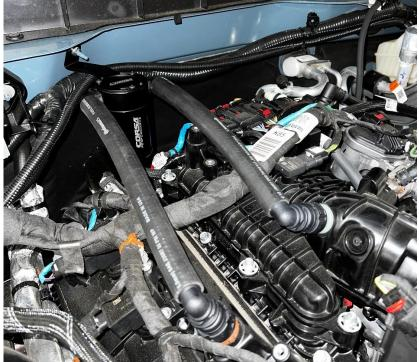
3. Install quick disconnect fittings to one end of each hose. Attach hose A (longer hose) to the "A" end of the catch can and route the hose to connect it to the BROWN fitting on the engine. Connect Hose B to the "B" side of the catch can and route the line to connect it to the WHITE fitting on the engine. Make sure fittings are fully secured and the hose is pushed all the way over the ends of the fittings.
