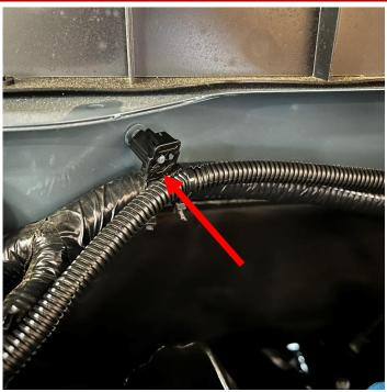
Located on the passenger side of the firewall, cut the zip tie securing the wiring harness to the plastic cap, then remove the plastic cap from the firewall stud.
