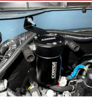
Use the provided nut and a 10mm socket wrench to secure the catch can in place on the firewall stud.
