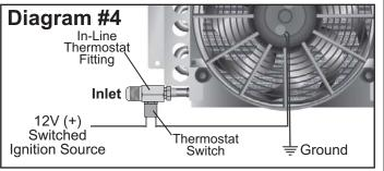
Warning: If this wire is connected directly to the vehicles battery the Electric Fan will run after the vehicle has been shut off.
