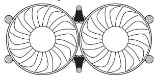
Dual fan mount using nylon tie rods
