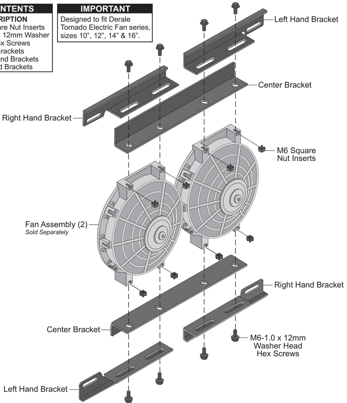
1. Slide 2 (two) each M6 Square nut inserts into slotted openings into position in flat landings on each end of electric fan assemblies as shown in illustration.
